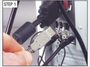
Simply connect the mountable extension cable once to the USB port on the back of your computer.
