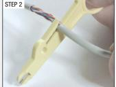
Remove approximately 3" of the outer jacket from the cable. Take care not to nick the wires.
