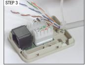
Secure the cable with a cable tie to the desired entry point.
