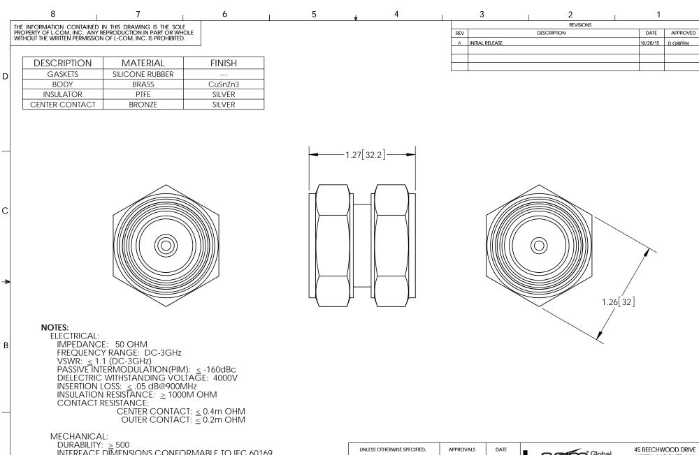
INTERFACE DIMENSIONS CONFORMABLE TO IEC 60169
