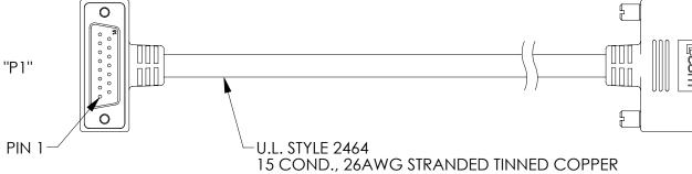
WITH ALUM/POLY FOIL SHIELD AND DRAIN WIRE JACKET: PVC, LIGHT GRAY, (PANTONE 400C)
