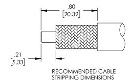
UNLESS OTHERWISE SPECIFIED LEADING DIMENSIONS ARE INCHES DIMENSIONS IN [] ARE MILLIMETERS
