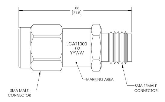
UNLESS OTHERWISE SPECIFIED LEADING DIMENSIONS ARE INCHES DIMENSIONS IN [] ARE MILLIMETERS TOLERANCES: .X=± .2 [5.08] **FRACTIONS** .XX=± .01 [.25] ± 1/32 XXX=± .005 [ .13 ] ANGLES ± 1°
