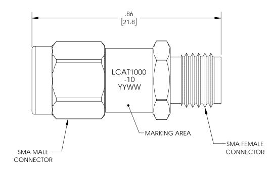
UNLESS OTHERWISE SPECIFIED LEADING DIMENSIONS ARE INCHES DIMENSIONS IN [] ARE MILLIMETERS TOLERANCES: .X=± .2 [5.08] **FRACTIONS** .XX=± .01 [.25] ± 1/32
