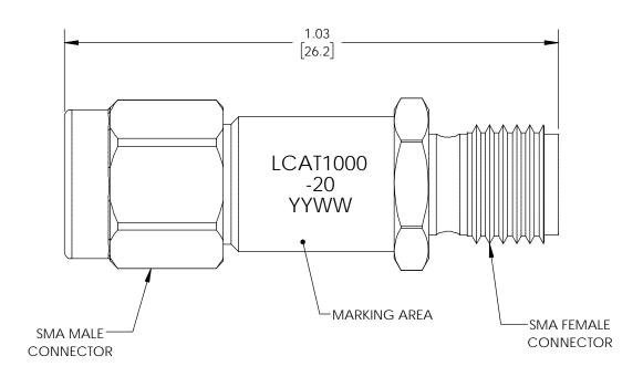
UNLESS OTHERWISE SPECIFIED LEADING DIMENSIONS ARE INCHES DIMENSIONS IN [] ARE MILLIMETERS TOLERANCES: .X=± .2 [5.08] **FRACTIONS** .XX=± .01 [.25] ± 1/32
