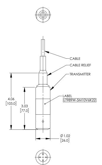
UNLESS OTHERWISE SPECIFIED LEADING DIMENSIONS ARE INCHES DIMENSIONS IN [] ARE MILLIMETERS TOLERANCES: an INFINIT® brand .X=± .2 [5.08] FRACTIONS 50 High Street, West Mill, 3rd Floor, Suite #30 .XX=± .01 [.25] ± 1/32 North Andover, MA 01845 USA. .XXX=± .005 [ .13 ] ANGLES ± 1° Phone: 1.800.341.5266 | 1.978.682.6936 ALL DIMENSIONS SHOWN ARE FOR REFERENCE ONLY. Fax: 1.978.689.9484 THIRD-ANGLE PROJECTION SIZE CAGE DRAWN BY **⊕** }
