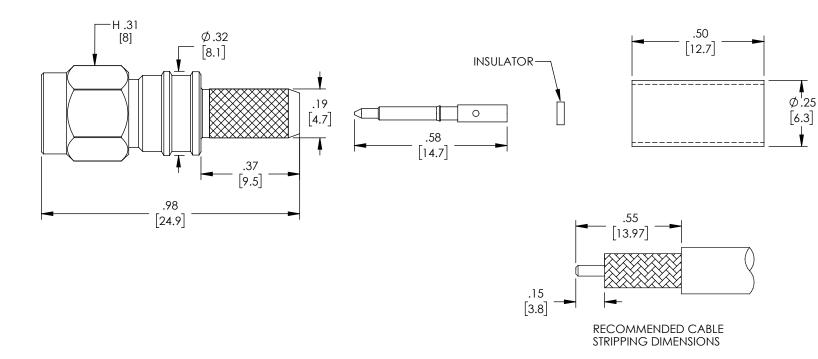
UNLESS OTHERWISE SPECIFIED LEADING DIMENSIONS ARE INCHES DIMENSIONS IN [] ARE MILLIMETERS
