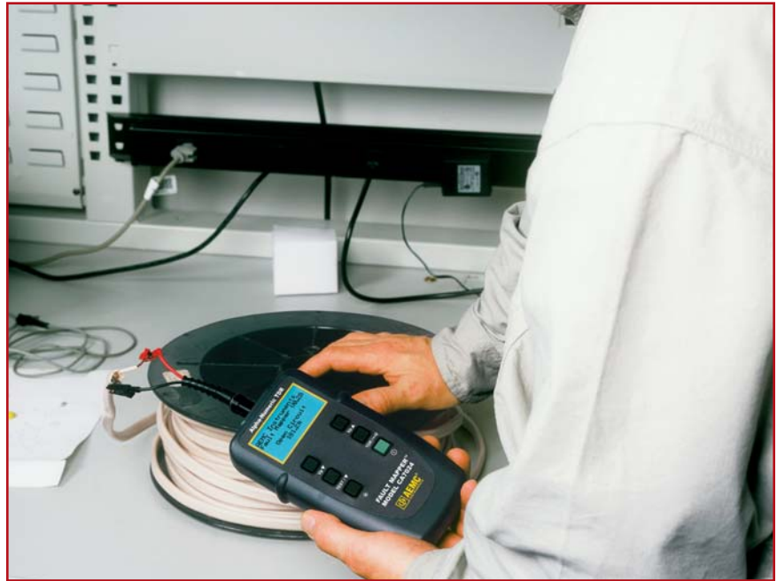
Model CA7024 checking the length of cable on a reel.
