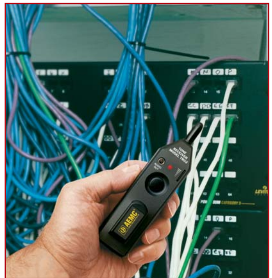
Model TR02 used to find cables in a panel.
