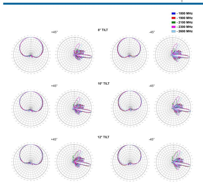
1710-2690 MHz, 65 Degree Sector Antenna, 18 dBi gain, 2-12 Degree RET, 4 x 4.3-10 Female Connector from L-com has same day
