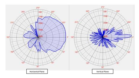
2300-2700/5150-5850MHz, 16 / 18 dBi, Wifi MIMO Sector Antenna, 90-degree, +/-45 Dual Pol, 2-Port, Type N Female Connector from
