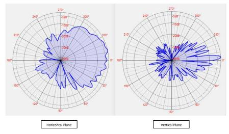
2300-2700/5150-5850/5900-7200 MHz, 16 / 18 / 17 dBi, Wifi MIMO Sector Antenna, 90-degree, +/-45 Dual Pol, 4-Port, Type N Female
