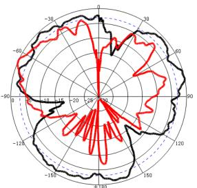
Freq:6000MHz Date:2016-05-19 Elevation:H-plane Polar-Across:Main Polarization:Vertical Max:-49.60dB HPBW(3dB):26.40° FBR:0.91dB Circularity:13.82
