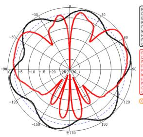
Freq:3700MHz Date:2016-05-19 Elevation:H-plane Polar-Across:Main Polarization:Vertical Max:-33.77dB HPBW(3dB):35.04\* FBR:0.33dB Circularity:3.88
