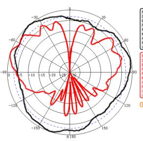
Freq:5500MHz Date:2016-05-19 Elevation:H-plane Polar-Across:Main Polarization:Vertical Max:-41.65dB HPBW(3dB):70.15\* FBR:0.13dB Circularity:3.00
