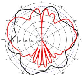
Freq:4900MHz Date:2016-05-19 Elevation:H-plane Polar-Across:Main Polar-Across:Main Polar-Across:Main Polar-Across:Max-36.67dB HPBW(3dB):29.20\* FBR:0.66dB Circularity:4.95
