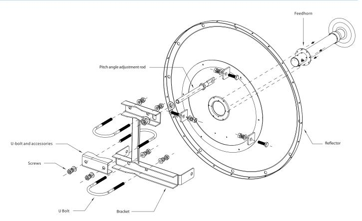
4950 MHz to 7125 MHz, 2-foot Parabolic Antenna, 2x2 MIMO, 30 dBi, RPSMA, 2 Pack from L-com has same day shipment for domestic and International orders. Our portfolio includes coaxial cable assemblies, connectors, adapters and custom products as well as lightning and surge protectors, NEMA rated enclosures, and an RF product line which includes antennas, amplifiers, passive, and active components.
