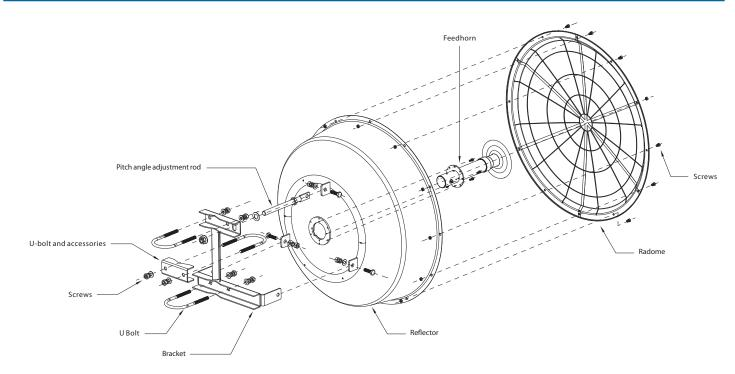
4950 MHz to 7125 MHz, 2-foot deep dish Parabolic Antenna, 2x2 MIMO, 30 dBi, RPSMA from L-com has same day shipment for domestic and International orders. Our portfolio includes coaxial cable assemblies, connectors, adapters and custom products as well as lightning and surge protectors, NEMA rated enclosures, and an RF product line which includes antennas, amplifiers, passive, and active components.
