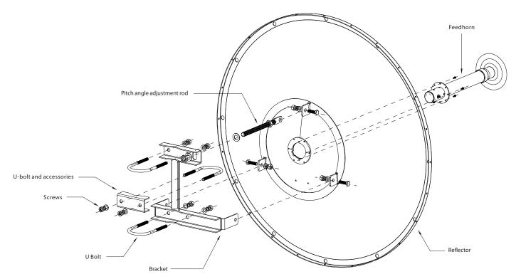
4950 MHz to 7125 MHz, 3-foot Parabolic Antenna, 2x2 MIMO, 34 dBi, RPSMA, 2 Pack from L-com has same day shipment for domestic and International orders. Our portfolio includes coaxial cable assemblies, connectors, adapters and custom products as well as lightning and surge protectors, NEMA rated enclosures, and an RF product line which includes antennas, amplifiers, passive, and active components.
