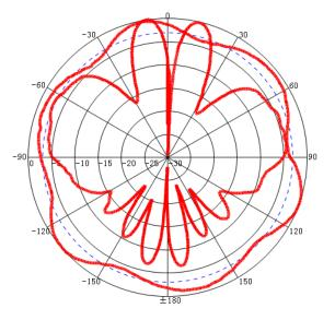
Freq:5500MHz Date:2015-10-09 Elevation:H-plane Polar-Across:Main Polarization:Vertical Max:-35.52dB HPBW(3dB):37.08\* FBR:0.90dB Circularity 2.32
