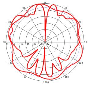
Freq:4900MHz Date:2015-10-09 Elevation:H-plane Polar-Across:Main Polarization:Vertical Max:-31.62dB HPBW(3dB):41.79\* FBR:1.00dB Circularity:2.77
