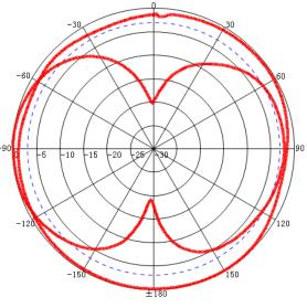
Freq:827MHz Date:2015-03-24 Elevation:V-plane Polar-Across:Main Polarization:Vertical Max:-12.73dB HPBW(3dB):88.93\* FBR:0.00dB Circularity:12.87 Obliquity:1.70\*
