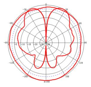
Freq:2700MHz Date:2015-03-24 Elevation:H-plane Polar-Across:Main Polarization:Vertical Max:-35.69dB HPBW(3dB):360.00° FBR:0.00dB Circularity1.34
