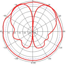
Freq:2200MHz Date:2015-03-24 Elevation:H-plane Polar-Across:Main Polarization:Vertical Max:-33.44dB HPBW(3dB):360.00\* FBR:1.37dB Circularity:1.18
