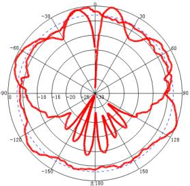
Freq:6000MHz Date:2015-10-09 Elevation:H-plane Polar-Across:Main Polarization:Vertical Max: 44.73dB HPBW(3dB):29.84\* FBR:3.10dB Circularity:3.28
