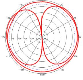
Freq:698MHz Date:2015-03-24 Elevation:H-plane Polar-Across:Main Polarization:Vertical Max:-11.05dB HPBW(3dB):360.00° FBW(1.18dB Circularity1.23
