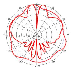
Freq:5800MHz Date:2015-10-09 Elevation:H-plane Polar-Across:Main Polarization:Vertical Max:-41.37dB HPBW(3dB):34.60\* FBR:2.43dB Circularity:2.65
