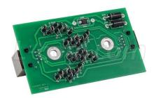
The unit features a low capacitance diode array that can withstand large surge currents. The design utilizes a Thyristor diode which switches to a low impedance state once triggered. This offers superior power handling capability compared to TVS or Zener diode based designs. The limits are +/- 58 volts on the four cable pairs.
