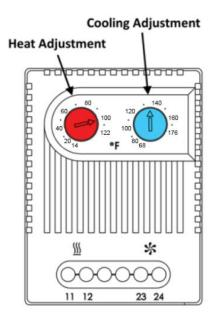
The cooling thermostat features a Normally Open (NO) circuit. When the temperature rises to the temperature set on the cooling adjustment dial the circuit closes which turns on the cooling fans. When the temperature falls below the temperature set on the cooling adjustment dial the circuit opens which turns off the cooling fans.
