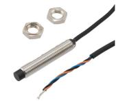
Inductive Proximity Sensor, cylindrical, M8 threaded, non-shielded, stainless steel, NPN NO, sensing distance 2mm, 2m 3-wire cable
