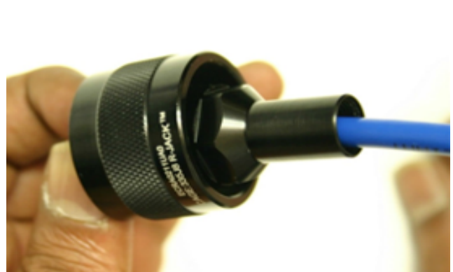
9.15 At this point locate the dust cap and place lanyard loop over RJ-45 plastic plug and wedge assembly .Locate the plug and slide the RJ-45 jack into the rear of the plug body. Bring the rear cap up towards the plug body and only screw them hand tight.
