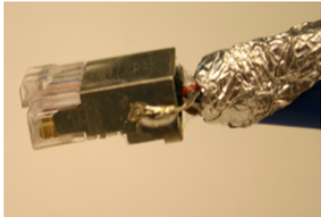
9.13 The RJ-45 plug body should look like this with the drain wire soldered and excess wire removed. The plastic hook should look like this as well.
