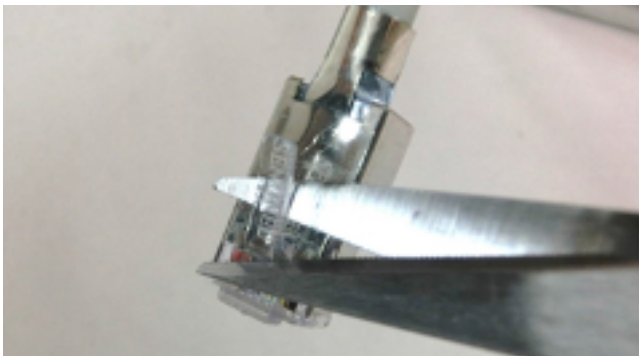
9.18 Cut off the plastic hook on the RJ-45 connector.
