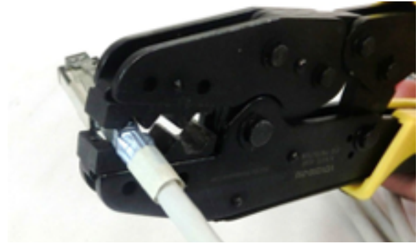
9.15 Crimp the back of the RJ-45 with a .255 hex crimp die. (shielded only)
