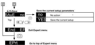
Some menu won't be shown depends on the setup. It's not a malfunction. Time of pressing buttons to activate not specified on this manual is 0.3 seconds. When the parameter value is ready to set, sub display will blink. Following parameters of the 2 output type (D3RF-TDM/S) can be specified individually for Output 1 (ch1) and Output 2 (ch2). Other parameters are specified commonly. Threshold, Output mode, Timer and its value, Teaching menu
