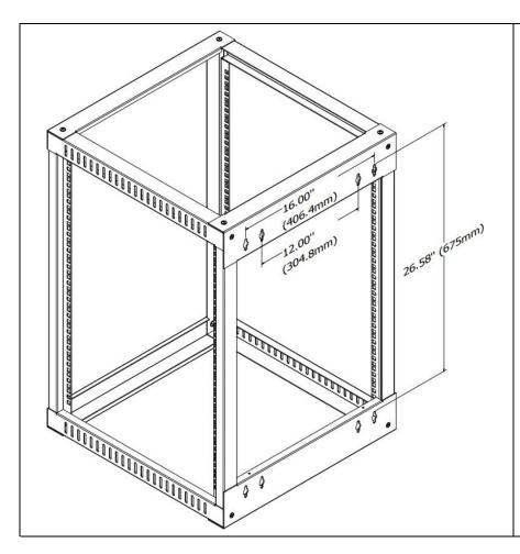
Attach the enclosure to a wall or other suitable mounting surface using appropriate anchors. The included Anchors (G) are intended for use on a concrete wall. The mounting holes are spaced 16" (406.4mm) and 12" (304.8mm) as reflected the diagram. in Warning: Do not attempt to mount to wall when equipment is already mounted inside the rack. The rack can hold up to 90 pounds evenly distributed. Make sure the wall surface can hold both the weight of the cabinet and the rackmounted equipment.
