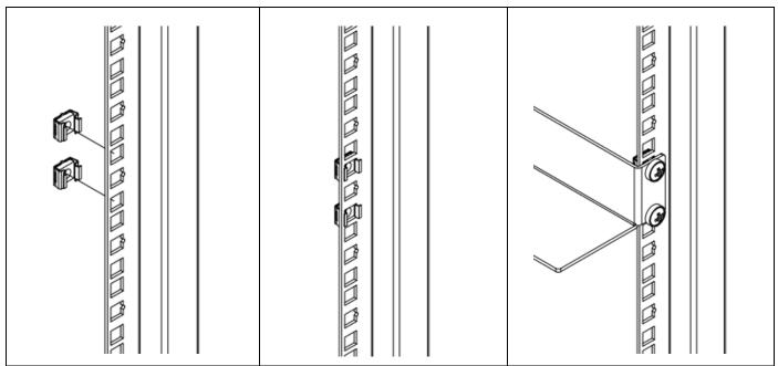
1. Locate the numbered square openings in the mounting rails where you plan to install your equipment. You will install cage nuts (included) into the square openings to provide an attachment point for the mounting screws (included).
