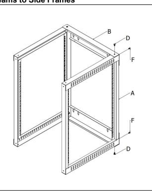
Attach both Back Horizontal Beams (B) to the Side Frames (A) and secure them with 4 of the M6\*12mm Screws (D), 4 of the M6 Flat Head Screws (F) and 8 of the M6 Flange Nuts (E) using a Phillips Screwdriver.
