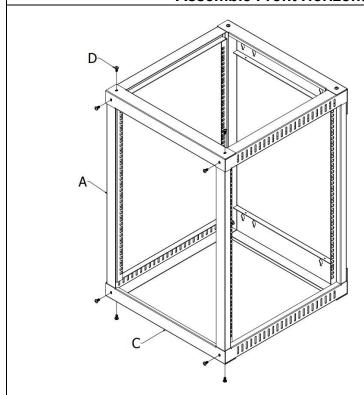
Attach Both Front Horizontal Beams (C) to the Side Frames (A) and secure them with 8 of the M6\*12mm Screws (D) and 8 of the M6 Flange Nuts (E) using a Phillips Screwdriver.
