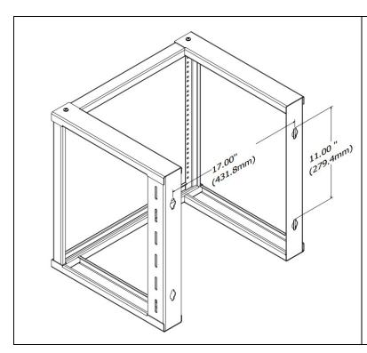
Attach the rack to a wall or other suitable mounting surface using appropriate anchors. The mounting holes are spaced 17" (431.8mm) as reflected in the diagram.
