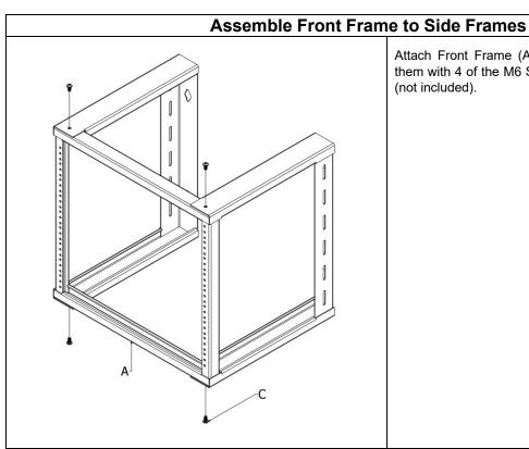
Attach Front Frame (A) to the Side Frames (B) and secure them with 4 of the M6 Screws (C) using a Phillips Screwdriver (not included).
