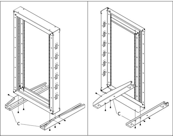
Attach Bottom Support Beams (C) to Frame with 8 of M6 x 12mm Screws (E) and 8 of M6 Flange Nuts (I) using a Phillips Screwdriver (not included).
