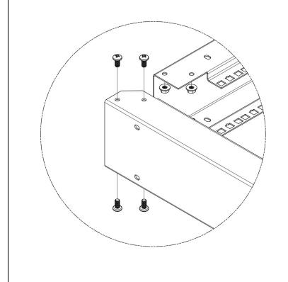
Insert the Vertical Rack Rails (B) into the Top/Bottom Cross Bars (A) and secure them with 16 of the M6 x 12mm Screws (F) and 16 of M6 Flange Nut (J) using a Phillips Screwdriver (not included).
