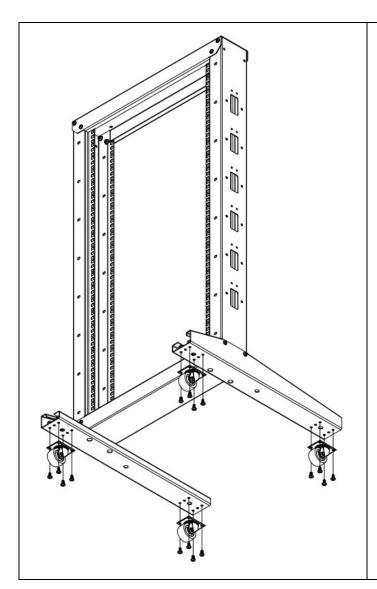
Attach 4 Casters (D) to each of the Bottom Support Beams (B) using 4 of M6 x 12mm Screws (E) and 4 of M6 Flange Nuts (I) for each Caster using a Phillips Screwdriver (not included) – NOTE: each support beam should have 1 Caster with Brake.
