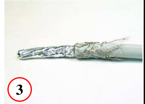
3 Fold outer shielding and drain wire back over cable jacket
