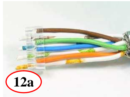
Trim Even wires 2, 4, 6, & 8 flush with bottom of Management Bar and insert
