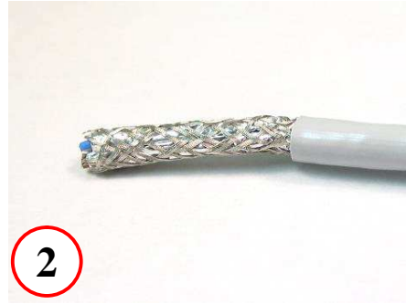
2 Strip off approx. 1" of cable jacket
