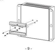
Step 2: Lightly press the bottom of DIN-rail bracket into the
