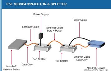
The PoE Injector provides DC voltage over Ethernet cable to power PoE devices, such as the splitter shown above. Th PoE Splitter divides the power and data signals from the cable, allowing the devices to operate within a PoE based network.
