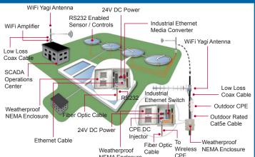
Includes WiFi antenna system, cable and CPE unit. A weather-proof NEMA enclosure contains an Industrial Ethernet switch, CPE DC injector and fiber optic cable. Network components include fiber optic, RS232 and Ethernet cables, along with media converters, power supplies and server drivers.
