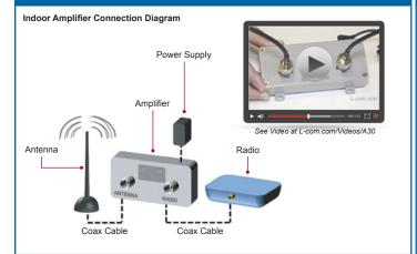
Low loss coax cable connects amplifier to the radio, in indoor and outdoor (using an enclosure) applications, for this WLAN communications network.
