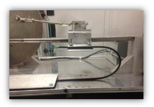
Flex cycling was performed for a desired time interval (i.e. 1M or 10M flex cycles)
