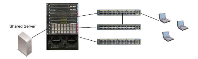
OSPF uses an algorithm that selects the shortest open path between routers. The laptop users above are in different IP subnets, each with different IP addresses. In order to communicate with shared resources (i.e. printers/servers) as well as the WAN via the core router, Layer 3 routes must be established. OSPF will determine the best, fastest route to those resources. Each OSPF router maintains routing tables of all other OSPF routers for best route determination.
