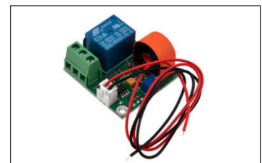
AC Current Sensor & Short Circuit Protector
